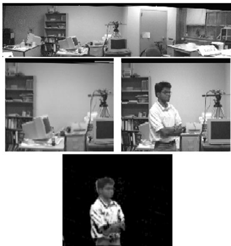
Fig. 3. Top image shows a panoramic background image mosaic constructed using a set of background images. The next row shows two images where the right image is a frame captured for the current pan and tilt position, and the left image is the corresponding background image indexed from the mosaic. The bottom image shows the segmented foreground object.
